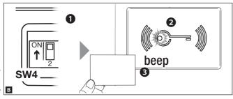
To remove badges from the associated relay, position DIP2 to ON ①. When the red LED on module MTMRFID starts to flash quickly ② swipe all the badges to be removed on the reader.
