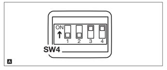
To restore module MTMRFID to factory settings it is necessary to disconnect the power supply, position DIP1 and DIP2 of SWITCH SW4 to ON and power the module again .
