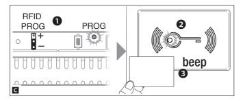
To remove badges, put the RFID PROG jumper of the power supply in the "-" position ①. When the red LED on module MTMRFID starts to flash slowly ②, swipe the badges to be removed on the reader twice.
