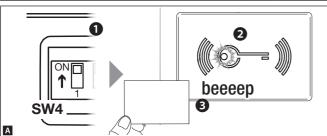
To associate badges with the selected relay, position DIP1 to ON ①. When the red LED on module MTMRFID starts to flash slowly ② swipe the badges to be associated on the reader ③.
