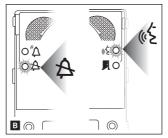
To associate badges, put the RFID PROG jumper of the power supply in the "+" position. The PROG LED on the power supply and LEDs ♣ and ﴿﴿É will flash quickly ▮ ▮.
