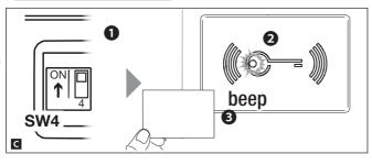
To remove lost badges, position DIP4 to ON ①. When the red LED on module MTMRFID stays constantly on ②, swipe all the badges previously acquired on the reader.
