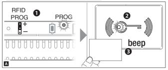
To associate badges, put the RFID PROG jumper of the power supply in the "+" position 1.
